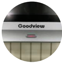
Power switch on front side
